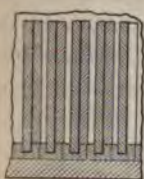
FIG. 2. ENLARGED SECTION SHOWING ANODES WITH DEPOSITED COPPER.
